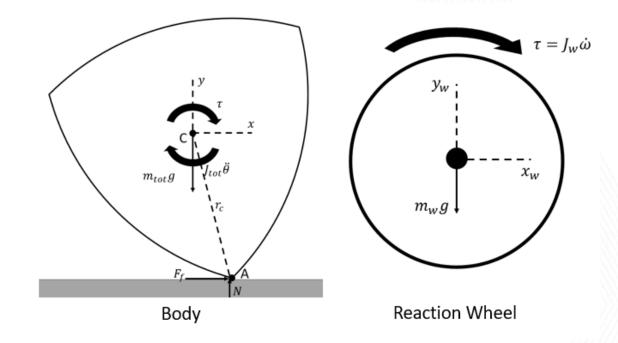
$$\frac{\Theta(s)}{V_{duty}(s)} = \frac{K_v(\frac{2\pi}{60})(J_w s)}{V_{max}(J_{tot}s^2 - m_{tot}gr_c)}$$
